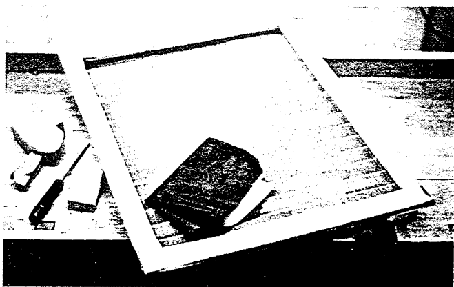
The deckle is fitted to a nearly completed mold.
